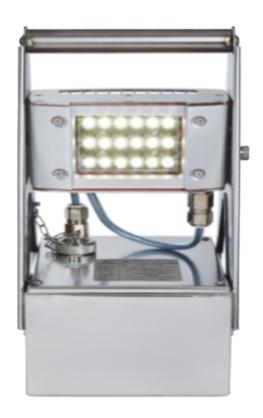
The Worklite™ is a rechargeable, high-output LED floodlight with ATEX, IECEx, and UKEX certifications. It is designed for harsh, remote environments, providing long-lasting light. It is CE marked for safe use in explosive gas, vapour, mist, and dust atmospheres in Zones 1, 2, 21, and 22, with a T4 temperature class.
