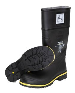
A heat-resistant safety boot conforming to the EN 15090 HI3 F3A fire boot standard for flame resistance, radiant heat (20kW/m2) and heat insulation of the sole (250oC for 40 minutes). These boots are designed for use in areas where there is a risk of sparks from welding or grinding or for close proximity fire fighting.
