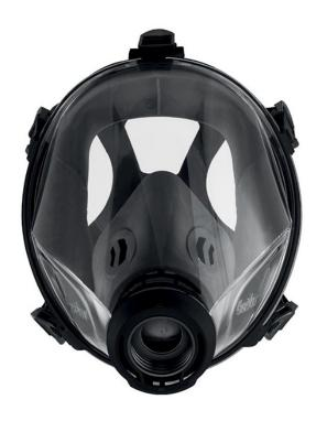
C 701 is the new full face mask of the Sèkur range which, through the innovative Air-On inspiration system, manages to combine a high protection factor with a minimum level of breathing resistance, assuring comfort and safety to the end user. C 701 can be used with particle, gas and combined filters equipped with EN 148/1 threaded connection, offering high protection against gases, vapours, solid and liquid particulates.
